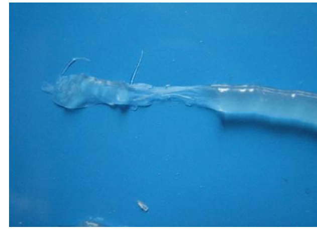
COHESION BREAK OF SILICONE SEALANT
